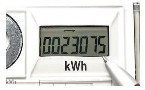
You should make a note of the first five figures on the digital display, but ignore the final figure if it begins with 0.1. You may need to press a button to get the reading to display.
