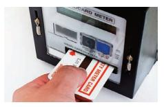
Prepayment meters are typically used in rented properties, or where households are struggling to pay bills or have built up debts in the past. The meters come with a single or two-rate reading, similar to that of Economy 7 meters. Read the figures from left to right, ignoring any red numbers.
