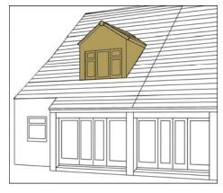
Fig 3. Dormers should be set back from the eaves line and the end or party walls
