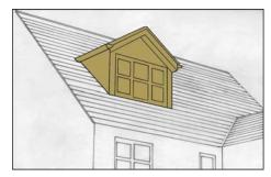
**Fig 2.** Dormers should appear subservient and be set lower than the ridge height of the existing roof. Dormers should also be proportionate, and not excessively bulky in relation to the rest of the roof.
