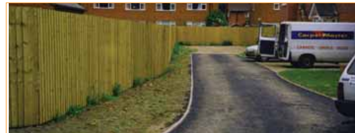
This poor quality close-boarded fence will require a high level of maintenance to ensure it provides a secure boundary
