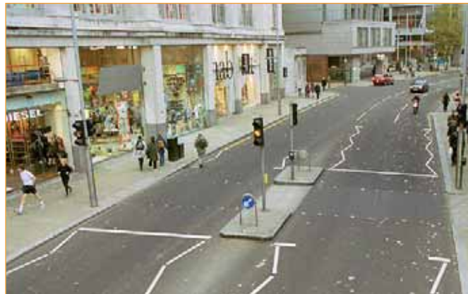
Above: This road carries four lanes of traffic, yet its pedestrian crossing is simple and uncluttered - making people on foot feel that they, too, are important.
