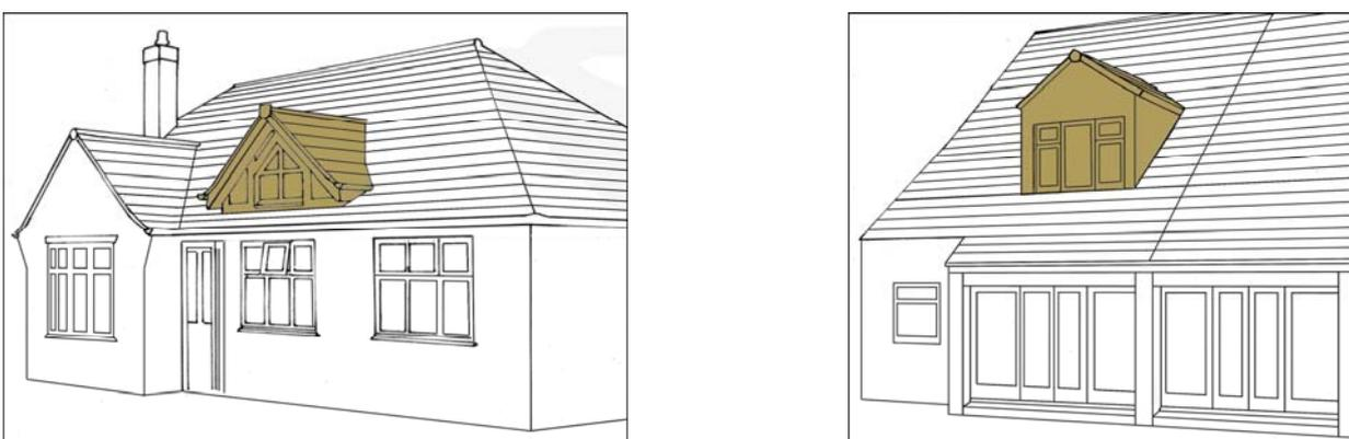
**Fig 3.** Dormers should be set back from the eaves line and the end or party walls
